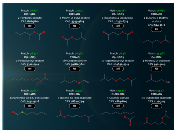
Figure 5: Identification of complex organics with PSG/MASS on laboratory samples. As a blind test experiment, the data were provided to us by Goddard’s Astrobiology Analytical Laboratory to determine its composition. We obtained the highest match (98.69%, right panel as shown by the retrieval web interface) with acetate 2-pentanol, consistent with the original source, while the model also identified several related species with similar structure and composition. The PSG/MASS search algorithm is extremely effective and fast (only taking ~1 second to obtain the results shown here), which enables rapid identification of complex species among a database of 21,000+ species at a broad range of masses and resolutions.
